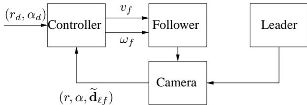
Fig. 3. Omnidirectional vision-based formation control scheme.
