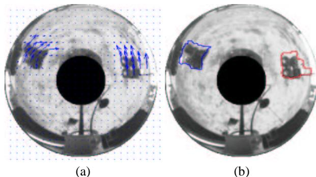
Fig. 1. Motion segmentation for two mobile robots based on their omnidirectional optical flows.
