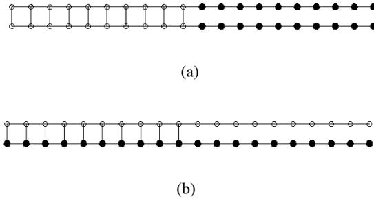
Fig. 4. The “roach” graph ( $n = 20$ ) illustrated here is a member of a family of graphs for which spectral partitioning is known to fail to produce a partition with low isoperimetric ratio. Uniform weights were used for both algorithms. (a) Solution using isoperimetric algorithm. Ratio = 0.1. (b) Solution using spectral algorithm. Ratio = 0.5.
