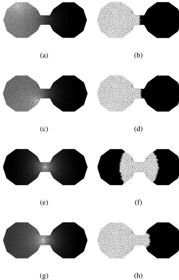
Fig. 3. An example of the effects on the solution with different choices of ground node for a problem with a trivial optimal partition. The left column shows the potential function (brightest point is ground) for several choices of ground while the right column shows thresholded partitions. Uniform weights ( $\beta = 0$ ) were employed.
