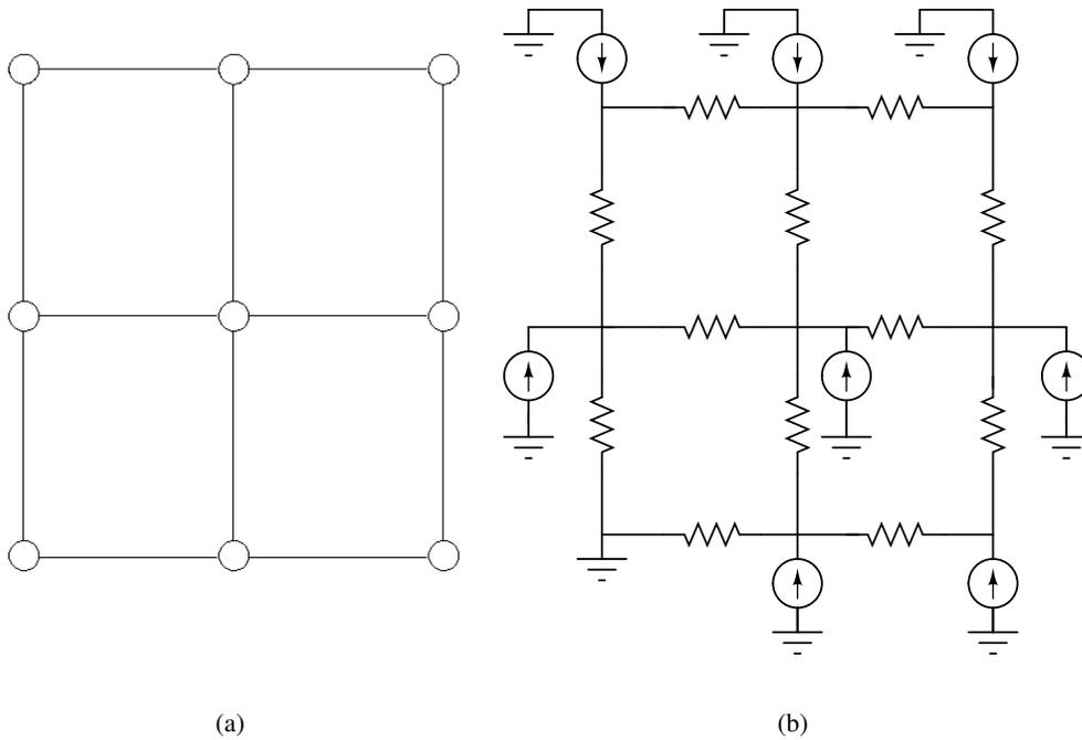
Fig. 1. An example of a simple graph and its equivalent circuit. Solving equation (16) (using the node in the lower left as ground) for the graph in (a) is equivalent to connecting the circuit in (b) and reading off the potential values at each node.
